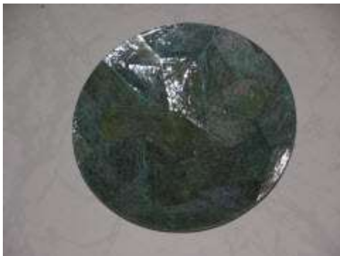
8" Plate, Abalone Cracking
